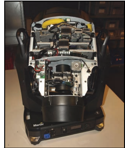
Figure 13: Head positioned for service access
