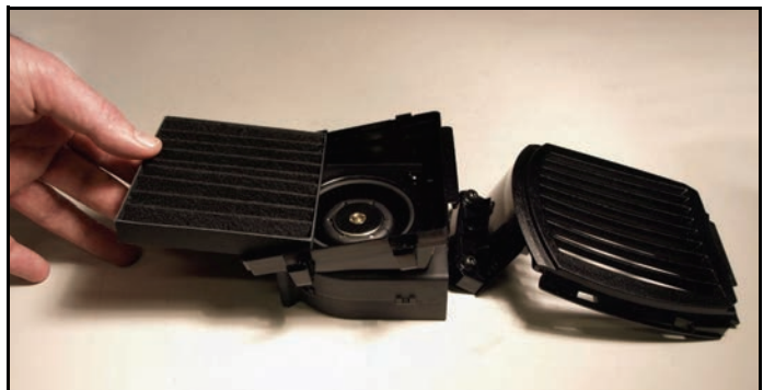
Figure 15: Head air filter alignment
