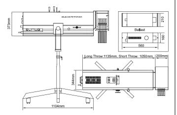
Luminaire Weight:25.5KgBallast Weight:23.4KgStand Weight:9.5KgColour Changer Weight:2.1Kg
