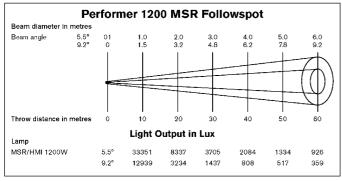
Tests conducted using a standard 1200W MSR/HMI single ended lamp.
